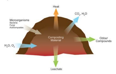
27. Composting is a biological process in which organic matter is broken down by aerobic (oxygen-requiring) microorganisms, such as bacteria, funghi and insects, which decompose the material in a controlled environment. Organic matter is first
